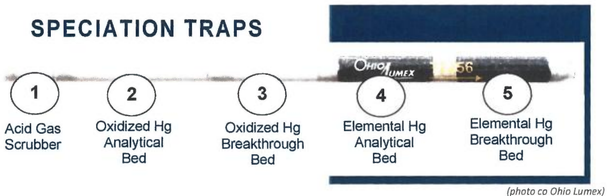
Figure 30B-2: Modified EPA 30B Speciation Sorbent Trap
